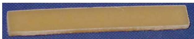
Figure 7 SLS specimen of PPC with 30% PTWs. [Color figure can be viewed in the online issue, which is available at www.interscience.wiley.com .]
